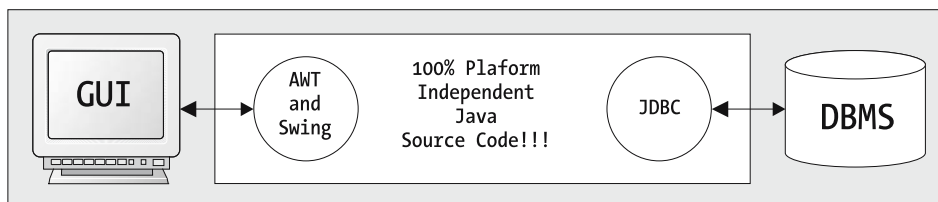
Figure 2-7. A 100% pure Java application is platform-independent from GUI to DBMS.
